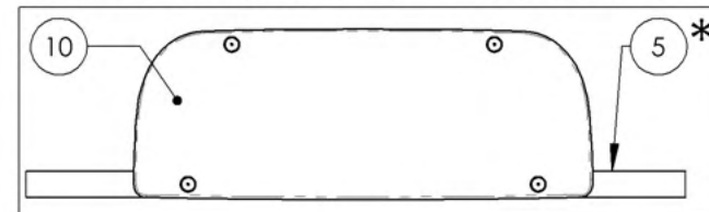
9003385 Footplate - Aluminium, Tubular Open Loop Structure, With ABS Cover, 12 x 4.75 in (Specify Wheelchair Serial Number)
