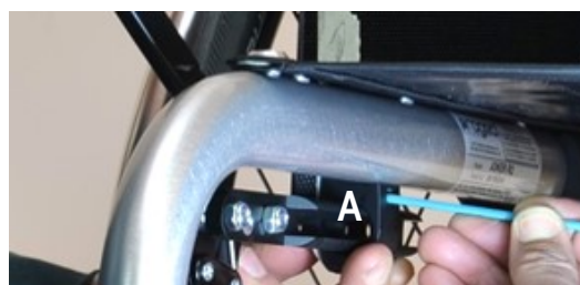
Mark the point where to drill the new hole
